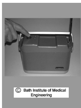
Figure 17 1-button radio: Radio can be turned ON/OFF with a single button
