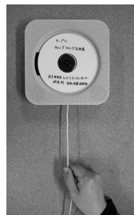
Figure 19 Wall-hanging CD player: CD player can be turned ON/OFF by pulling down the power code.
