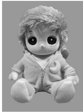
Figure 23 Talking doll: The dolls talks when the user touches the hand, etc. of the doll.
