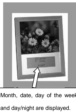
Figure 4 Automatic calendar (with time slot function): Month, date, and day of the week are displayed together with an eye-catching photo.
