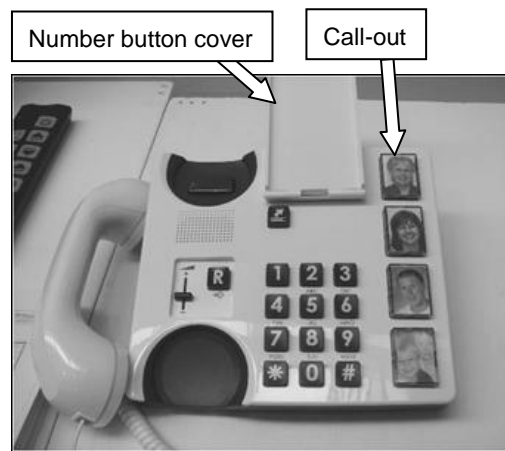
Figure 21 Simple phone with photo buttons: A cover for hiding number buttons is provided.
