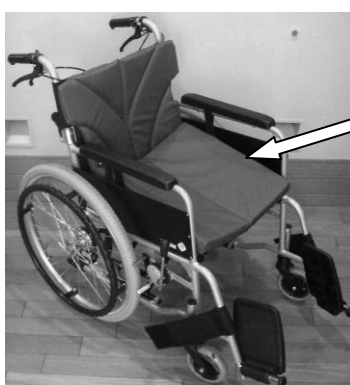
Figure 13 Wheelchair with automated brakes: When the user stands up, the seating surface will be raised and brakes will be applied.
