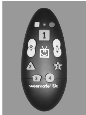
Figure 15 Simple TV remote controller (with different buttons) having five operation buttons with different shapes
