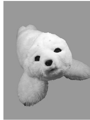
Figure 24 Seal-shaped communication robot: The robot responds by crying or moving the body if stroked or talked.
