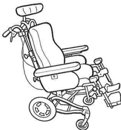
Figure 18 A wheelchair with a tilt mechanism and posture support devices
