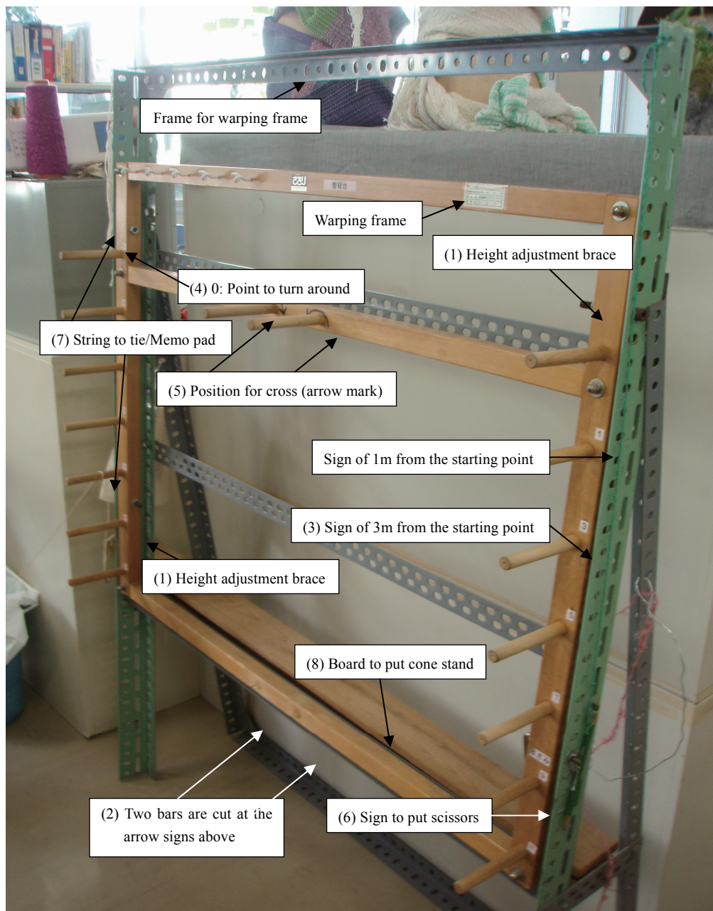
Figure 18. Warping frame and its frame (made by National Rehabilitation Center for Persons with Disabilities)
